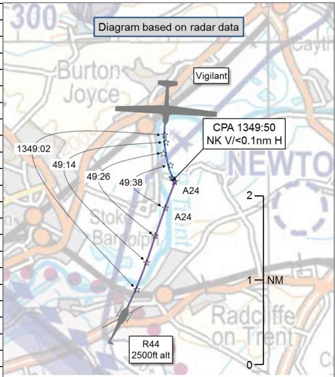
**THE VIGILANT (GROB 109) PILOT** reports that, whilst descending to rejoin RW20 at RAF Syerston, he completed two descending left-hand turns at approximately 10° angle of bank. Whilst passing through a heading of approximately 220°, and descending through 1800ft, he glanced right to see an R44 helicopter pass directly overhead by approximately 80ft. He immediately reported this to the Duty Instructor by RT.
